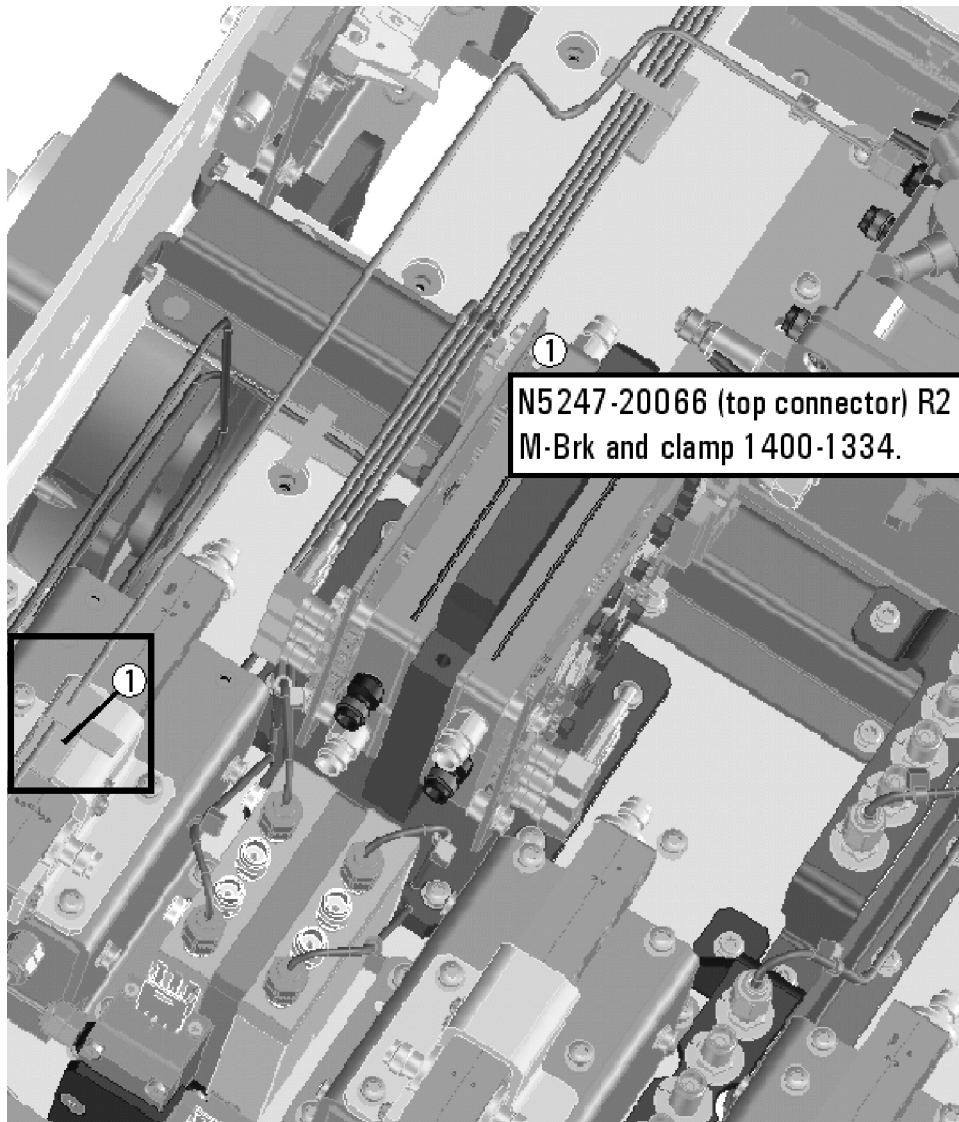
Figure 6 Location of Cable Clamp to Secure W145 (N5247-20066)
